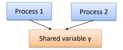
Loop forever I<sub>1</sub>: non-critical section while y<= 0 wait I<sub>2</sub>: y := y-1; I<sub>3</sub>: critical section y = y+1 ; End loop
